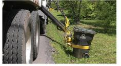
The **Command-SST** has a 3-axis arm that allows for above-grade and below-grade can access.
