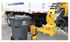
The **Command-SST** features a significant reduction in lubrication points, all in easy-to-reach locations at ground level.
