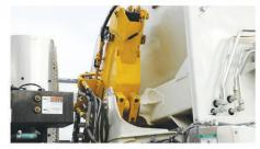
The body-mounted arm is easy to service and produces less cab rocking than other arms.
